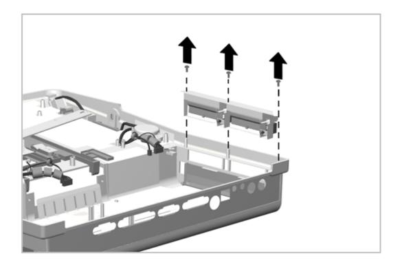
Figure 6-23. Removing the PC Card Door Assembly
